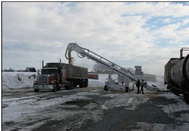
Before: Grain cars shared a siding with bio-fuel and lumber cars. There was no clean-up pad and capacity was limited to two spots. Center-beams were unloaded on grade crossings.
